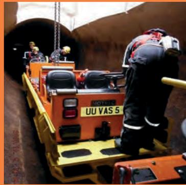
Left: The Vehicular Access System (VAS), provided safe access to the 8km of tunnel works
